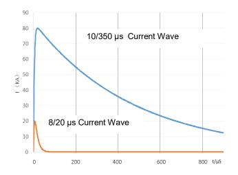
Standard lightning test wave
